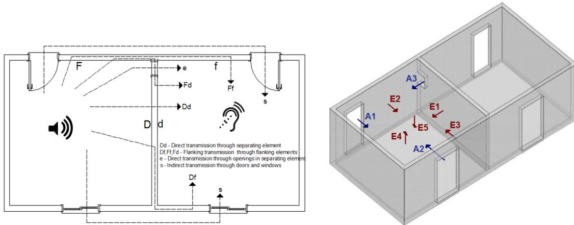
Figure 1: Definition of sound transmission paths between two rooms.
