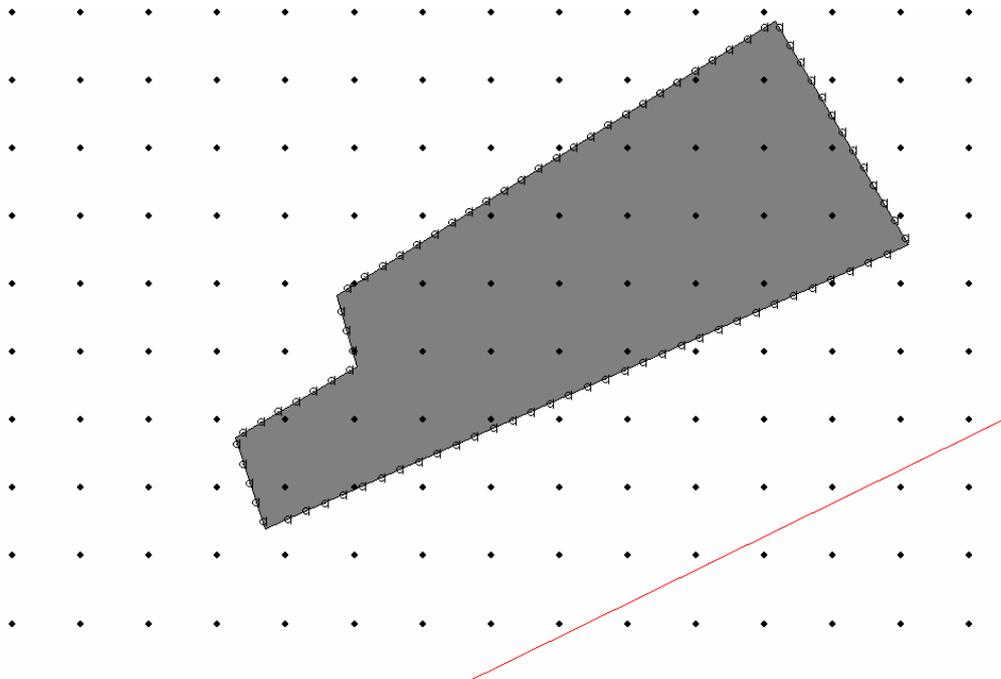
**Figure 17: The two options for calculating the noise levels reaching a dwelling (either applying a fine grid, either placing receivers on and around the dwelling's surfaces)**
