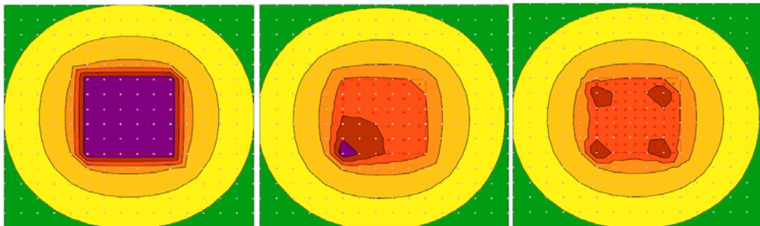
**Figure 13: Different results for the same area source with different selection of grid spacing (from left to right - 40\*40m, 37\*37m, 23\*23m)**
