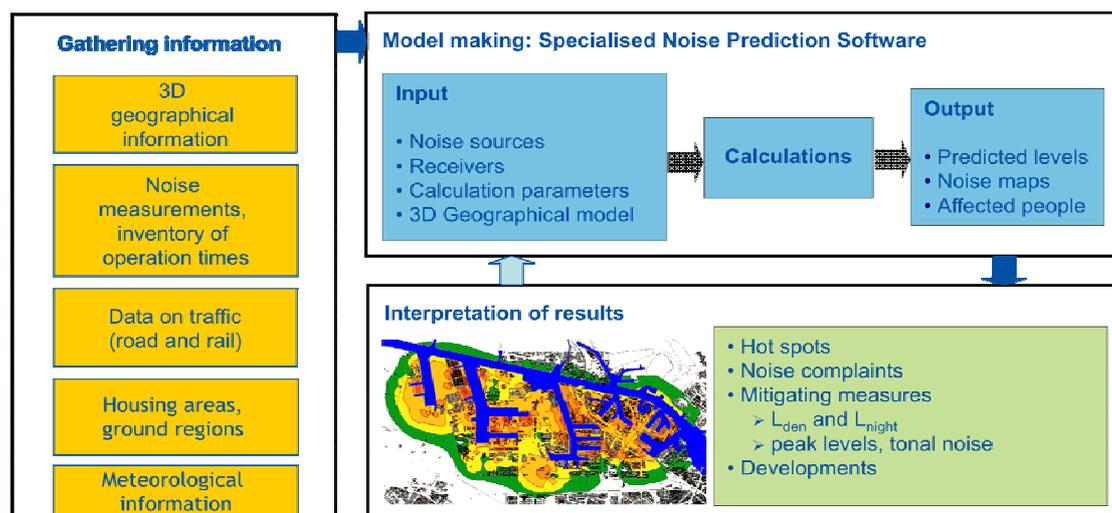
**Figure 6: General schematic function of a noise mapping task**
