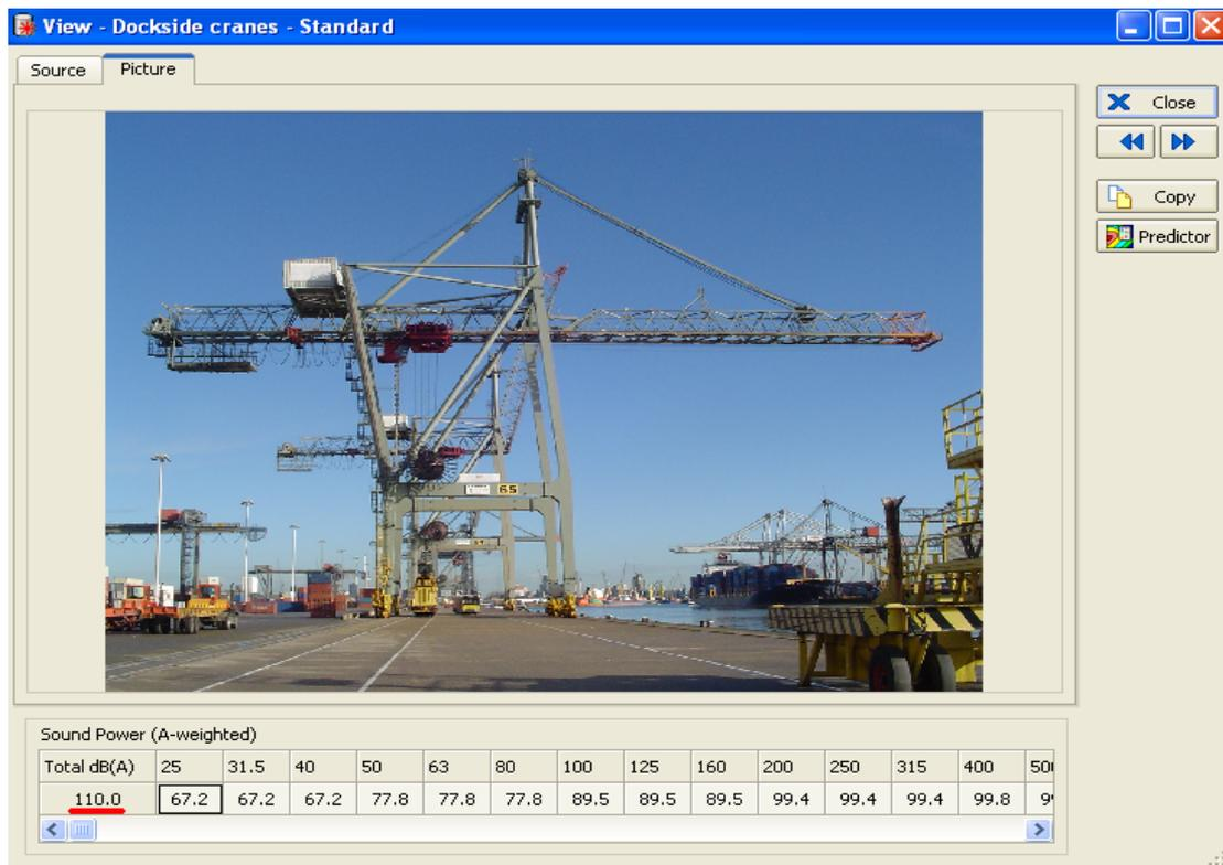
**Figure 10: The entry “dockside cranes” in the Imagine Source-dB Database**
